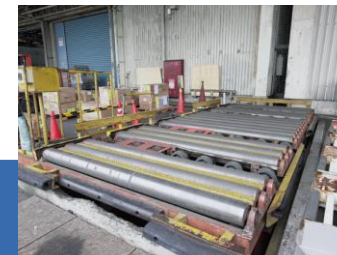
20 feet lifter Main Cargo : Unit Load Device (ULD)
