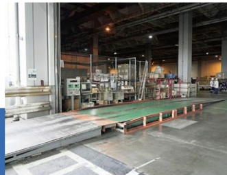
20 foot pit scale scale : 20ton
