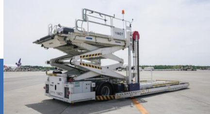
9 Main Deck Loader A vehicle for loading and unloading ULD from a freighter aircraft's main deck
