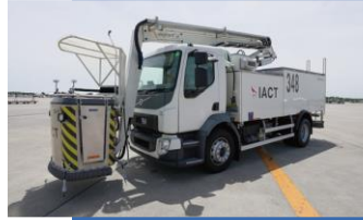
4 Deicing car A Vehicle for the removal of snow and ice from an aircraft
