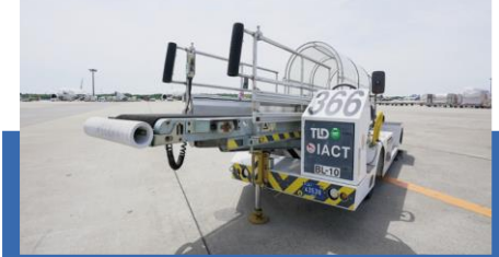
10 Belt Loaders A vehicle for loading and unloading bulk cargo and baggage from an aircraft's bulk cargo bay
