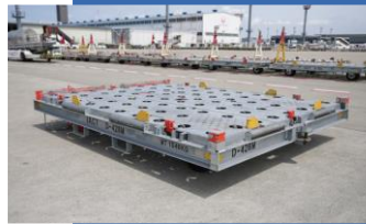
575 Pallet Dolly Equipment for transporting ULDs
