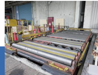
20 feet lifter Main Cargo : Unit Load Device (ULD)
