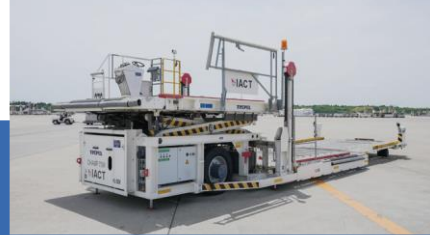
9 High Lift Loaders A vehicle for loading and unloading ULD from an aircraft's lower deck
