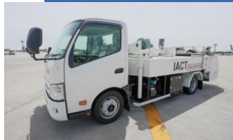
2 Lavatory Service Cars A vehicle for extracting wastewater, such as from aircraft lavatories, and transporting it to a treatment facility.
