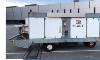
1 Air Start Unit Equipment for starting aircraft jet engines
