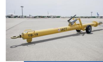
19 Tow Bar Stick-like equipment for connecting an aircraft to a towing car
