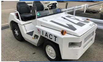
55 Towing Tractors A vehicle for towing ULD dolly and bulk cart
