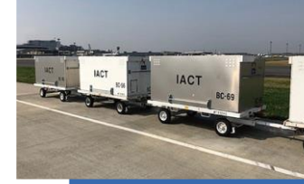
88 Bulk Carts Equipment for transporting bulk cargo and passenger baggage
